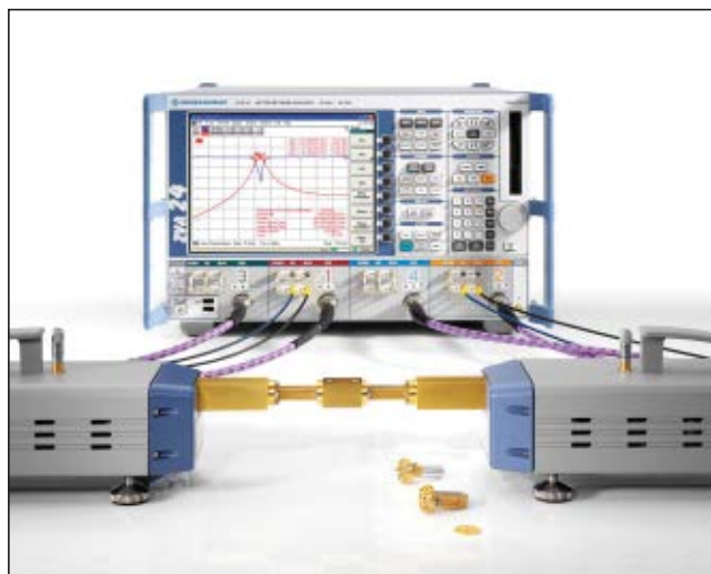
▲ Fig. 3 Complete millimeter-wave set up measuring a 90 GHz bandpass filter, together with the R&S ZV-WR10 waveguide calibration kit.
