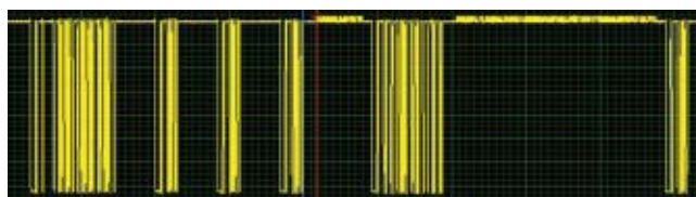
▲ Fig. 7 Symbol information for an ISO18000-6 Type C RFID query transaction acquired by a VSA and passed through the demodulation block.
