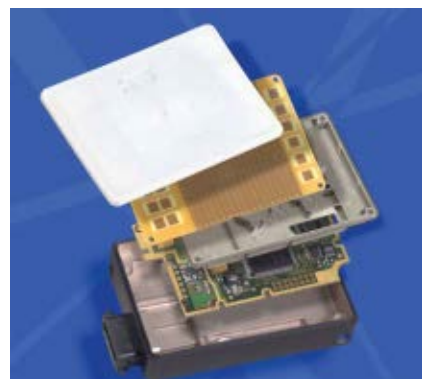
▲ Fig. 17 Exploded view of a 24 GHz UWB automotive sensor currently available in the US and EU. The unit is approximately the size of a deck of cards.
